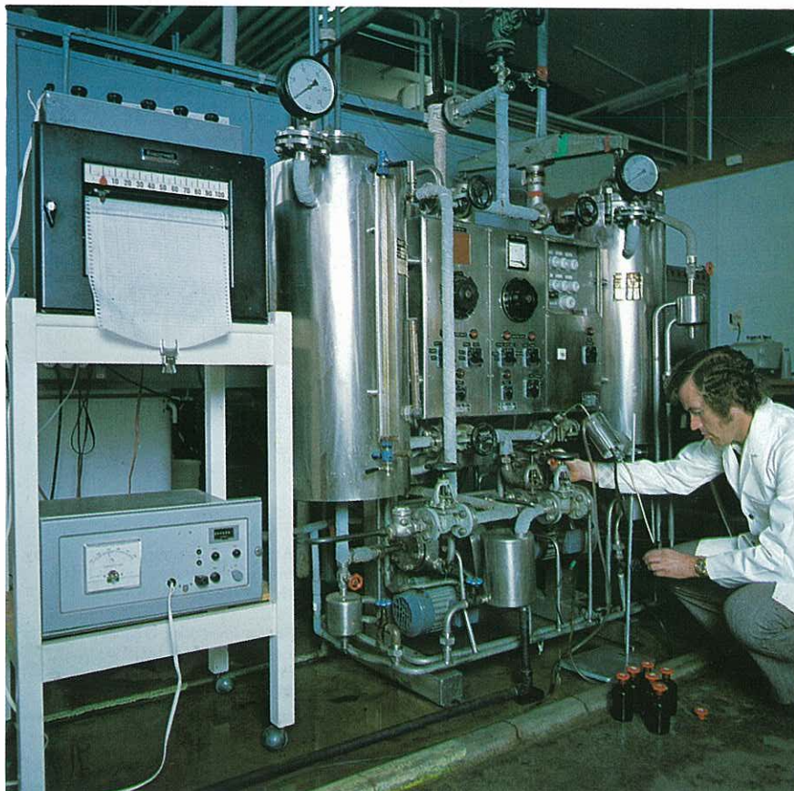
Sample of pulp liquor being taken from the laboratory batch digester during FRI experiments. (FRI CT119).
